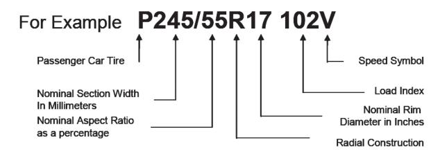
**Load Index Number**, a numeric code which indicates the maximum load carrying capacity of a tire at the maximum cold inflation pressure. Speed Symbol, an alphabetical code which indicates the maximum speed at which the tire can carry a load corresponding to its Load Index when properly inflated. These two items together are known as the "Service Description".
