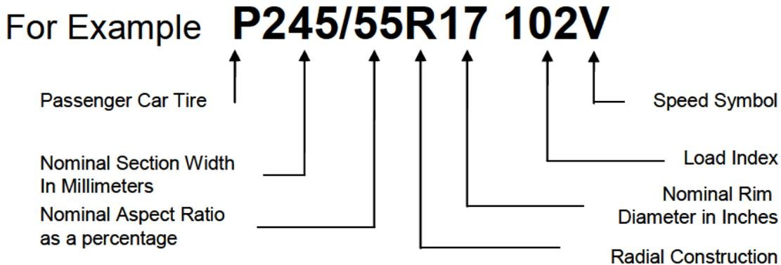
**Load Index Number**, a numeric code which indicates the maximum load carrying capacity of a tire at the maximum cold inflation pressure.
